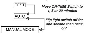
\* If you get confused while switching modes, turn the power off for one minute, then back on. After the calibration time the control will be in the AUTO mode.
